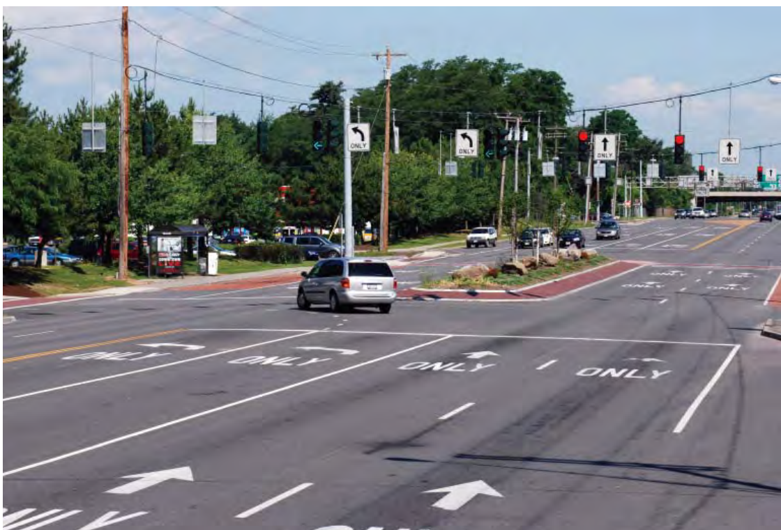
Figure 7-10. Urban Arterial with Dual Left-Turn Lanes
