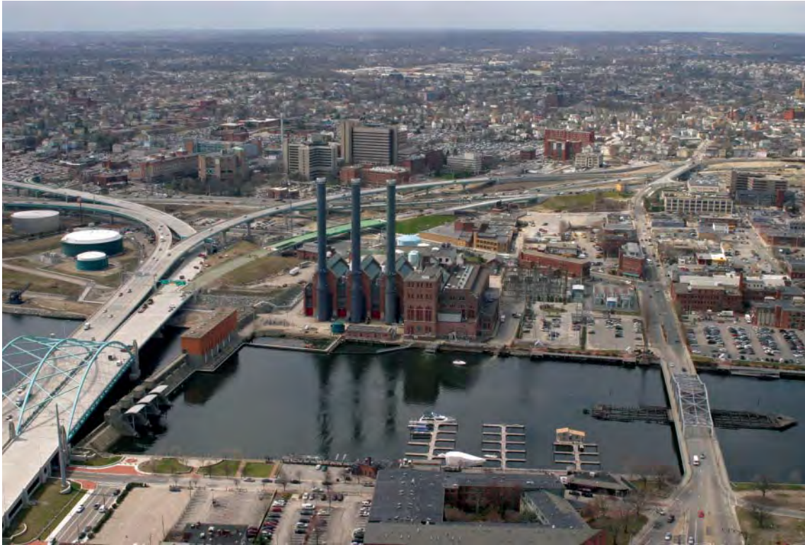
Figure 10-13. Directional Three-Leg Interchange at a River Crossing
