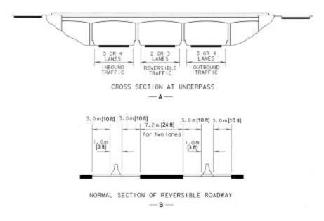
Exhibit 8-21. Typical Cross Sections for Reverse-Flow Operation
