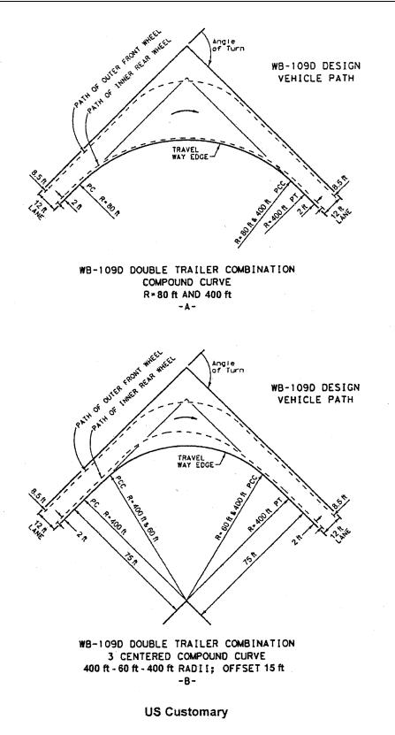
Exhibit 9-28. Minimum Edge-of-Traveled-Way Designs (WB-33D [WB-109D] Design Vehicle Path) (Continued)
