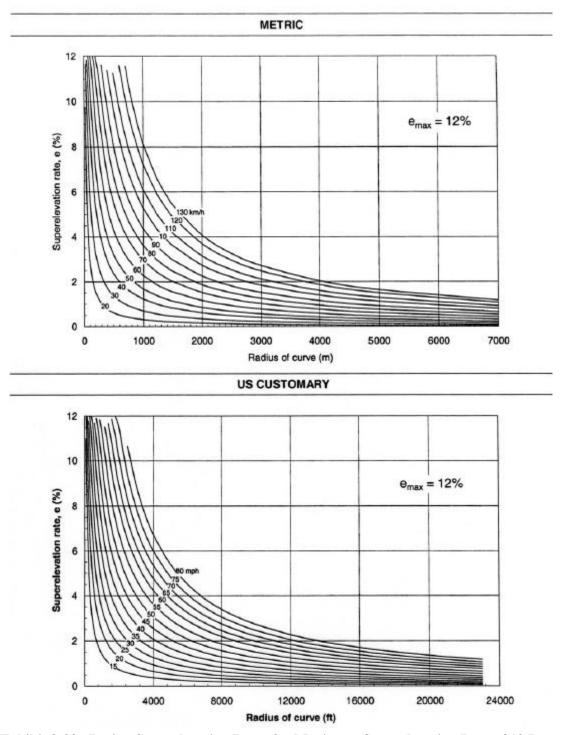
Exhibit 3-20. Design Superelevation Rates for Maximum Superelevation Rate of 12 Percent
