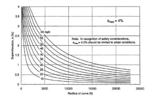
Exhibit 3-16. Design Superelevation Rates for Maximum Superelevation Rate of 4 Percent
