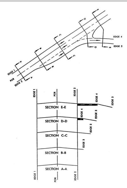
Exhibit 9-48. Development of Superelevation at Turning Roadway Terminals
