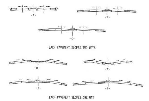
Exhibit 4-3. Roadway Sections for Divided Highway (Basic Cross Slope Arrangements)
