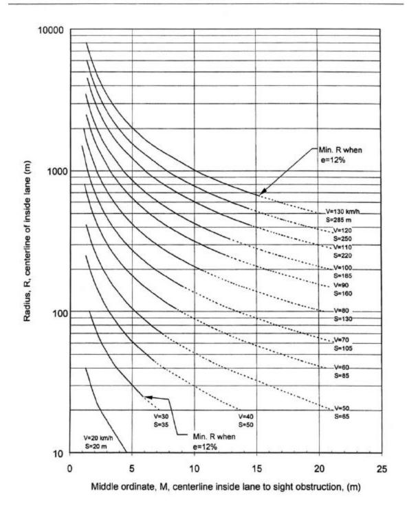
Exhibit 3-57. Design Controls for Stopping Sight Distance on Horizontal Curves
