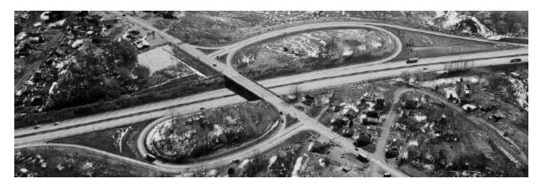
Exhibit 10-29. Four-Leg Interchange (Partial or Two-Quadrant Cloverleaf with Ramps Before Main Structure)
