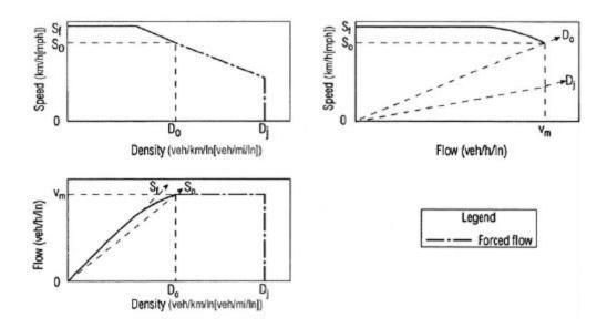
many vehicles on the roadway that flow has stopped. The maximum flow is reached at the point of maximum density.
