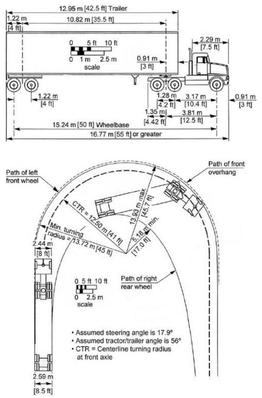
Exhibit 2-14. Minimum Turning Path for Intermediate Semitrailer (WB-15 [WB-50]) Design Vehicle
