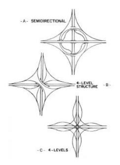
Exhibit 10-33. Semidirectional and Directional Interchanges—Multilevel Structures
