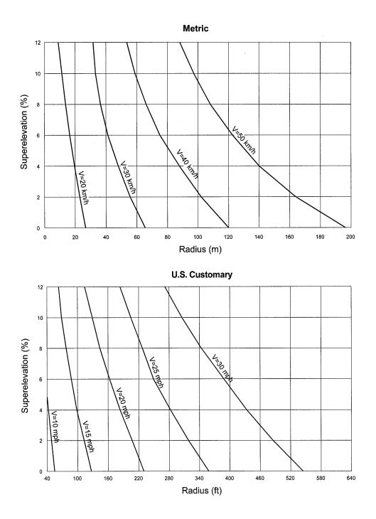
Exhibit 5-16. Minimum-Radius Horizontal Curve for Gravel Surface
