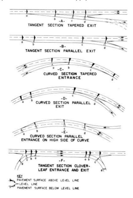
Exhibit 10-58. Development of Superelevation at Free-Flow Ramp Terminals
