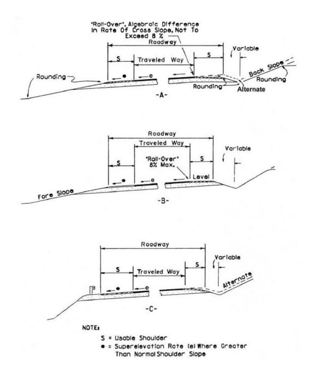
Exhibit 4-2. Typical Cross Section, Superelevated
