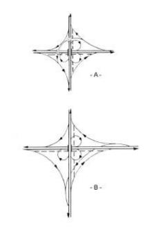
NOTE: WEAVING ADJACENT TO THE THROUGH LANES IS ELIMINATED BY PROVIDING COLLECTOR-DISTRIBUTOR ROADS AS SHOWN BY DOTTED LINES.
