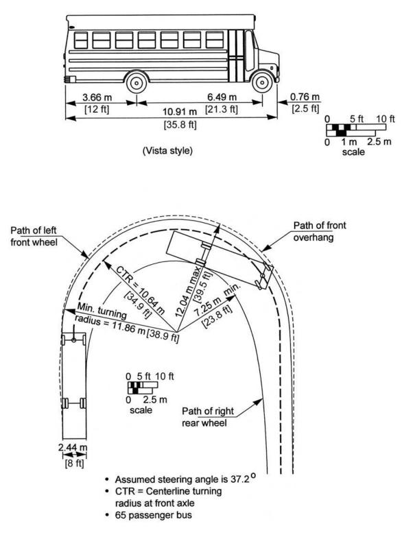
Exhibit 2-8. Minimum Turning Path for Conventional School Bus (S-BUS-11 [S-BUS-36]) Design Vehicle
