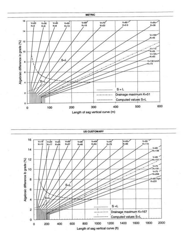
Exhibit 3-78. Design Controls for Sag Vertical Curves—Open Road Conditions
