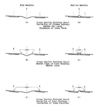
Exhibit 7-6. Methods of Attaining Superelevation on Divided Arterials
