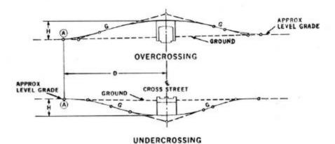
NOTE:"MINIMUM VERTICAL CLEARANCE SHOULD BE CHECKED UNDER THE OUTSIDE EDGE OF THE OVERCROSSING STRUCTURE"
