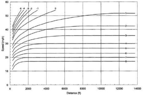
Exhibit 3-60. Speed-Distance Curves for Acceleration of a Typical Heavy Truck of 120 kg/kW [200 lb/hp] on Upgrades and Downgrades
