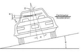
a = Ball Bank Indicator angle o = Body roll angle • = Superelevation angle
