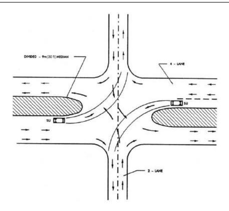
Exhibit 9-99. Four-Leg Intersection Providing Simultaneous Left Turns
