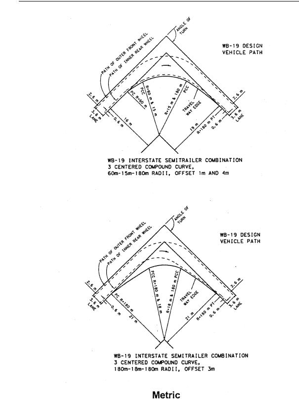
Exhibit 9-26. Minimum Edge-of-Traveled-Way Designs (WB-19 [WB-62] Design Vehicle Path)
