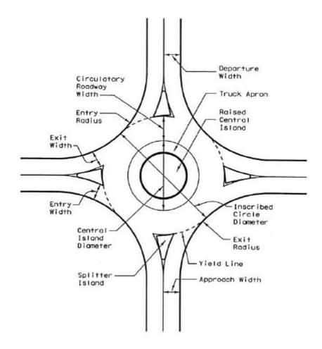
Exhibit 9-15. Geometric Elements of a Single-Lane Modern Roundabout
