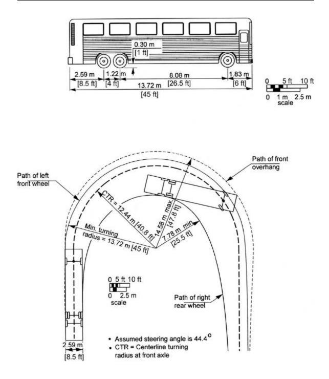
Exhibit 2-6. Minimum Turning Path for Intercity Bus (BUS-14 [BUS-45]) Design Vehicle
