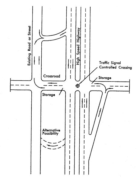
Exhibit 9-90. Special Indirect Left-Turn Designs for Traffic Leaving Highway with Narrow Median
