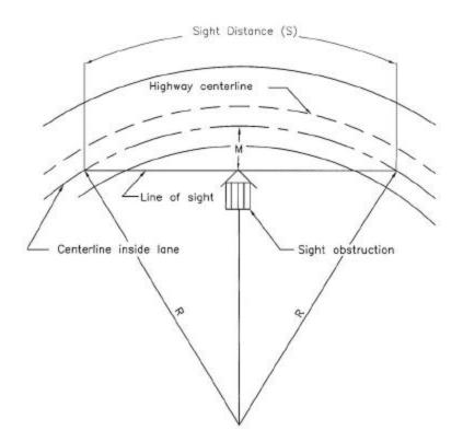
Exhibit 3-58. Diagram Illustrating Components for Determining Horizontal Sight Distance
