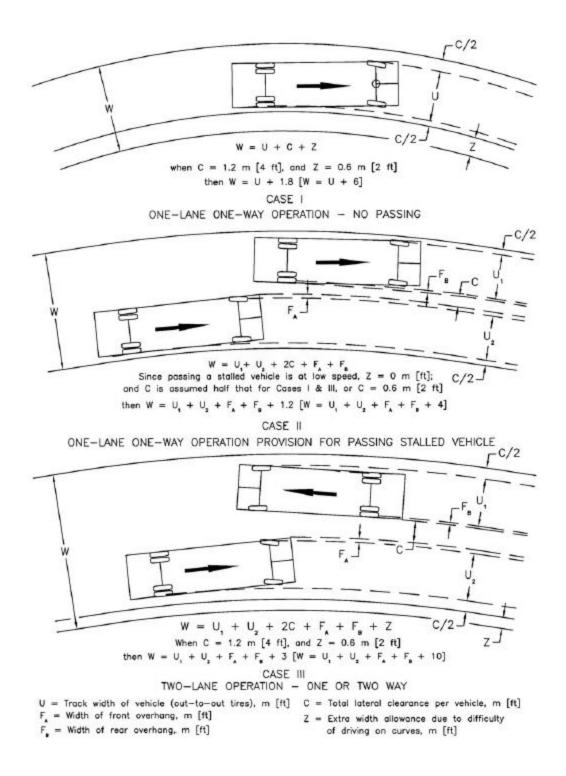
Exhibit 3-53. Derivation of Turning Roadway Widths on Curves at Intersections
