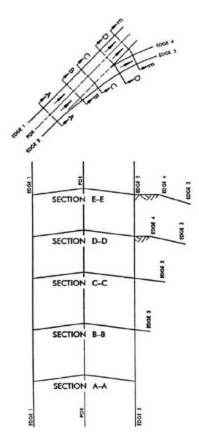
Exhibit 9-45. Development of Superelevation at Turning Roadway Terminals
