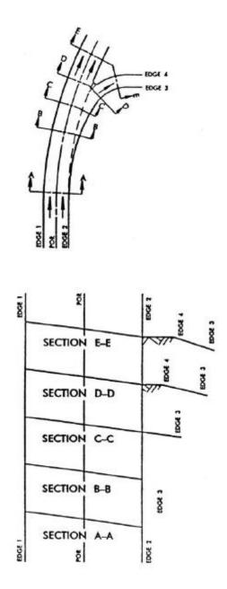
Exhibit 9-46. Development of Superelevation at Turning Roadway Terminals
