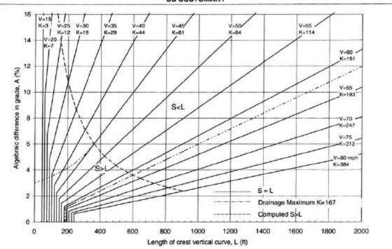
Exhibit 3-75. Design Controls for Crest Vertical Curves—Open Road Conditions
