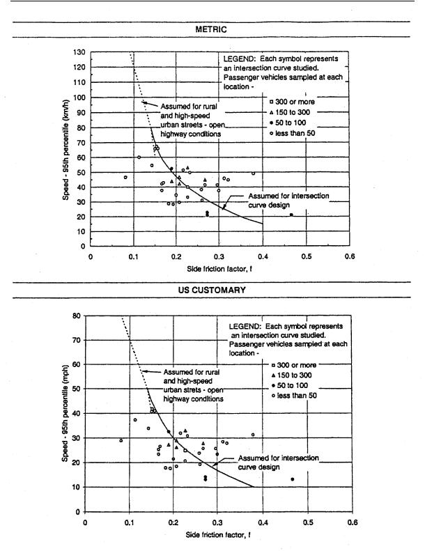
Exhibit 3-42. Relation Between Speed and Side Friction Factor on Curves at Intersections
