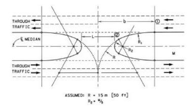
Exhibit 9-87. Above Minimum Design of Median Openings (Typical Bullet-Nose Ends)
